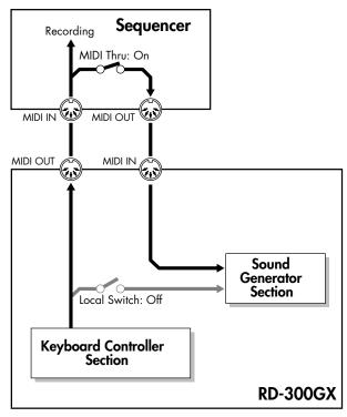
In this case, the data sent over two paths, i.e., the data sent directly from the keyboard controller section and the data sent from the keyboard controller section via the external sequencer, ends up being sent to the sound generator section simultaneously. Thus, for example, even when you play a "C" key only once, the note "C" cannot be sounded correctly, as the sound is played by the sound generator section twice.
